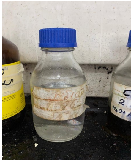
Figure no. 1 - The correct waste bottle for NITAL solution was faded and therefore it was difficult to be identified, therefore, the waste was accidentally put into the wrong bottle
